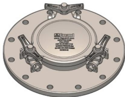
170mm Inspection 3 points, 6mm thickness, neckring depths 46mm ( Including the height of flange ) .Suitable for tanks with limited height space. Connected to the welding flange on the tank body through screw kits. Manlid seal and flange screw kits sold separately.
