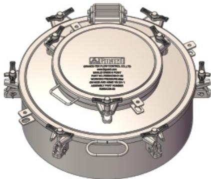
DN500 With stands 4Bar Pressure Manlid Assembly -With DN300 Inspection, when using PTFE coated EPDM seal ring, bolt locking torque up to 90N.m, pressure resistant 4Bar (25°C). manlid cover with inspection cover, save tank opening. It is suitable for the tank car whose detection pressure is 4Bar.
