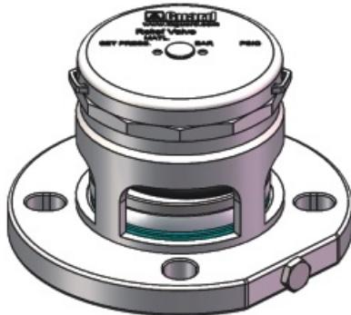
PFA Lined Safety Relief Valve are suitable for pressure ranges from 1.5 to 106.1 PSI (0.1 to 7.31 Bar) for pressure and from 0 to 3 PSI (0 to 0.21 Bar) for vacuum. The whole body is made of stainless steel, and the contact parts of the medium is lined with PFA, and the contact parts are made of PTFE. This kind of relief valve has strong anti-corrosion ability.
